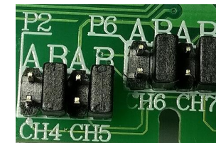
Thermistor: Pin B short
